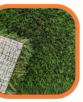
Colour Four tones green with brown and beige curl Roll Size 2m and 4m roll widths x 25m Composition Polyethylene and polypropylene Type C and Diamond Monofil **Dtex 14,300** Pile Height 30mm **Gauge 3/8"** Stitches/m<sup>2</sup> 14,175 Total Weight 2,615 g/m<sup>2</sup> **Primary Backing Polypropylene Secondary Backing Transparent latex** Permeability 175 I/min/m<sup>2</sup> (UNE-EN 12616:2014)
